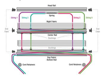
4.1 Remove screws from cord retainers at bottom of the window. Next remove shade from window
